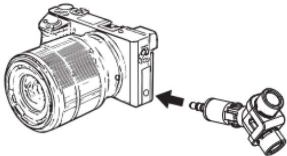
First Step: Insert Microphone into 3.5mm TRS socket
